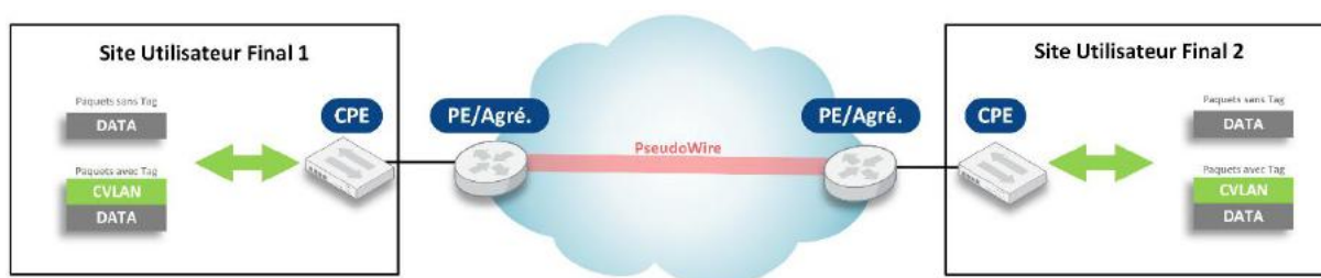
Figure 4 - Exemple de Topologie Lan-to-Lan
